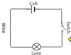
This circuit will not work because the switch is open. A circuit must be complete Switch have a battery/cell.
